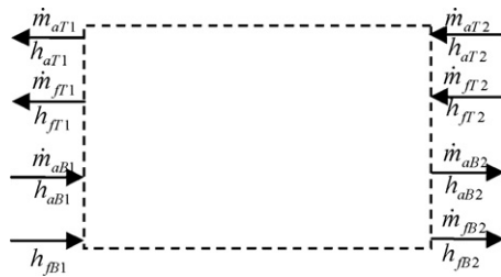
Fig. 13. Control volume of the desiccant wheel.
